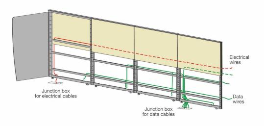
Slots provided on the frame vertical upright for passing of wires from one frame to other
