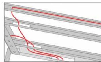
Cable flow at intermediate raceway level
