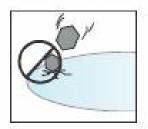
• Avoid any kind of impact on the glass surface as it may cause the surface to shatter / break / crack.
