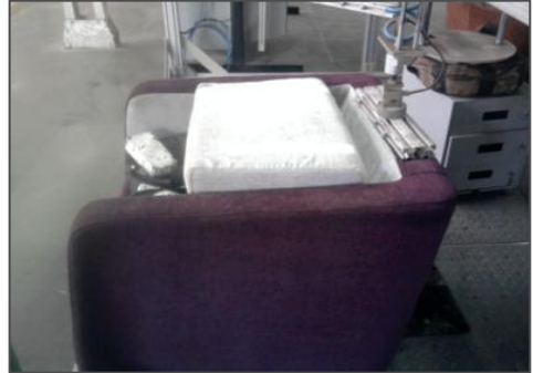
Backrest Strength Test - Horizontal Static & Vertical Static
