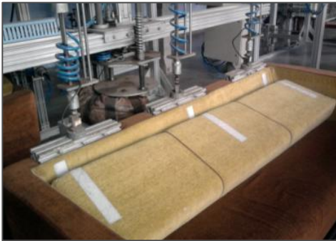
Backrest Strength Test – Vertical Cyclic
